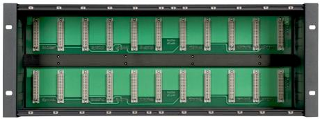
The 4U-high and 6U-high frames also use sliding nuts for the fixing of the modules. Please take care that the sliding nuts are moved to the correct position before you install a module. The pictures show a 4U-high frame with a collection of mastering modules and an empty 4U frame and an empty 6U frame with a power cable.
