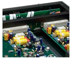
The above picture shows two 2U modules fixed to a spacer. This combination has exactly the same size as a 4U module. The other picture shows the motherboard in a 1U-high frame with two modules installed. The picture below shows a 1U-high frame without top cover sheet with partly removed modules. This picture demons-
