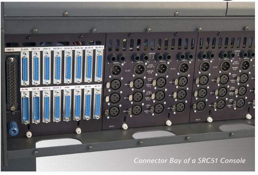
connector. Even though the pinning of all connectors is the same with all versions of the console. There are 15 25-pin female audio connectors and 2 25-pin male control connectors.
