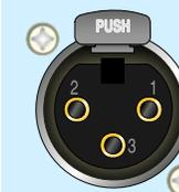
ALL SCREENING PINS ARE CONNECTED TO FRAME'S CONNECTOR-GROUND
