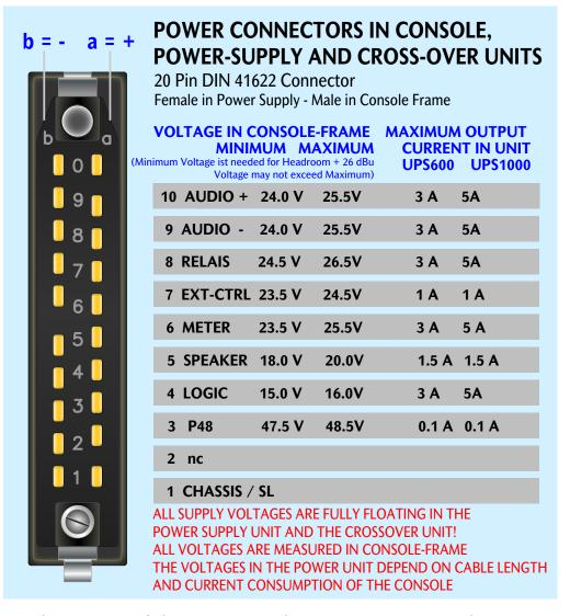
The pinning of the UPS600 and UPS1000 power supply units
