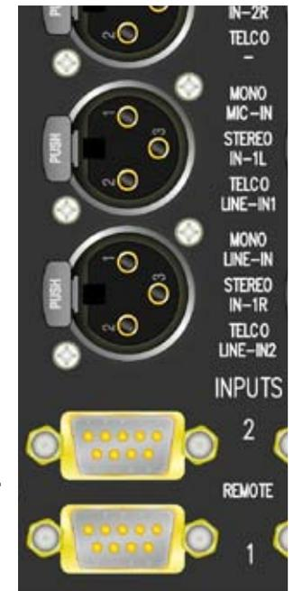
between pin 5 (+) and pin 9 (switched -). In addition, there are two, active low inputs for external switches. Both inputs are pulled to +24V. The switch current is less than 1mA. The inputs are protected against overvoltage. Both inputs are active when connected to Relay Ground.
