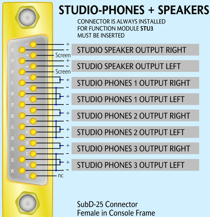
While the studio speakers outputs are standard, electronically balanced, line level outputs, the headphone outputs are unbalanced to drive headphones directly. Each output can drive approx. 3
